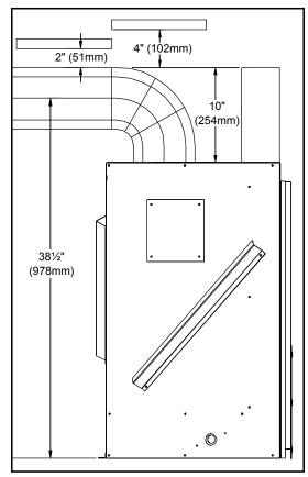
Figure 23. Hard Vent Pipe Clearances.
